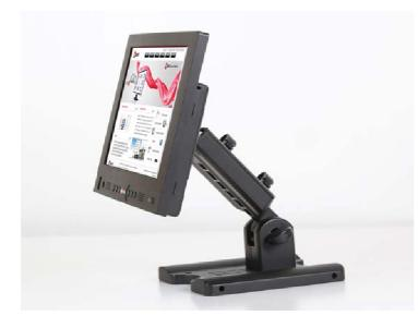
faytech's new 7-10" Touch Monitor Series sets new standards: HDMI port, three video inputs, extended current input (12-36V), extra robust components, exclusive design, mountable, Backlight LED, no pixel faults, high-quality pedestal, extended temperature range and suitable for 24/7operation are just some of the features that these monitors fulfill.
